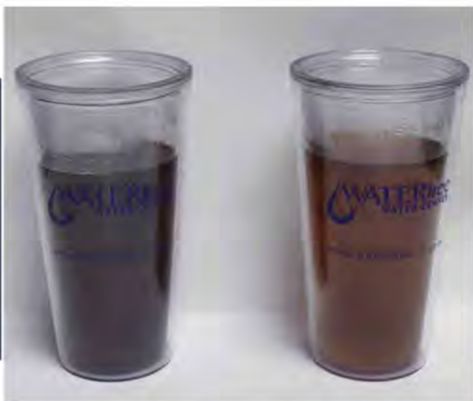
Iced Tea brewed for 5 minutes. The cup on the left was made with tap water with total dissolved solids (TDS) measuring at 800 while the cup on the right was made with reverse osmosis water with a TDS of 10.
